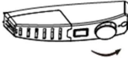
Your refrigerator has one control for regulating the temperature. The temperature control is located on the right side of the fridge.
